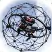
Drone used to perform pressure vessel inspections.
