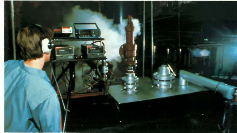
Pressure Relief Valve Under Steam Performance Test
