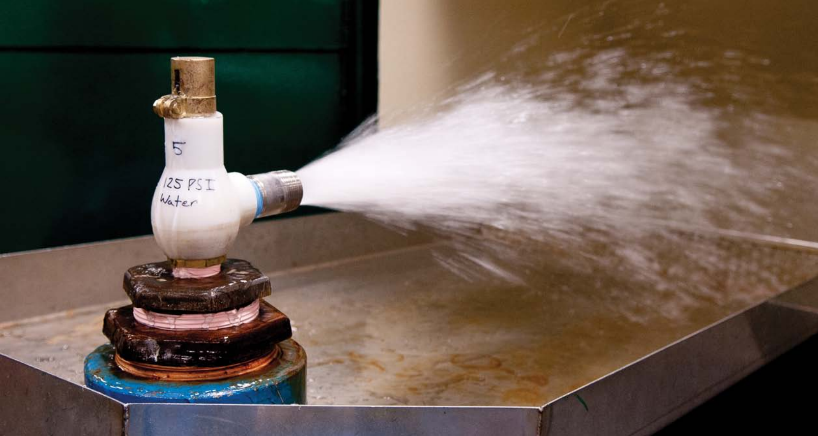
The National Board Test Lab's very first 3D printed valve part from F.C. Kingston, a liquid service PRV, undergoes successful water testing.
