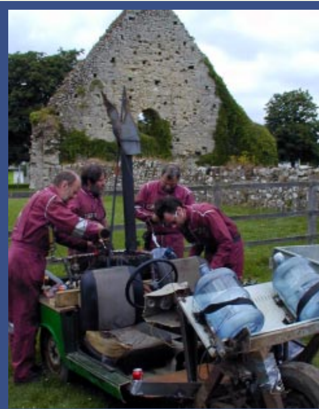
A CLOGGED INJECTOR: Crash works to clean “gunk” out of the injector while Richard tinkers with the boiler.
