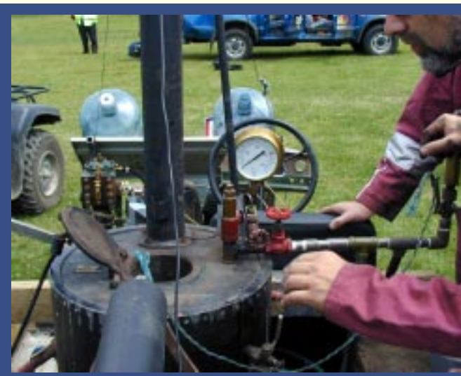
SMALL BUT POWERFUL: The pot boiler’s top-mounted firehole presented special challenges for Richard, the NERDS’ fireman.
