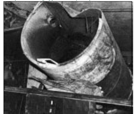
Where the boiler of the New York Telephone Co. came to rest after traveling approximately 120 feet.
