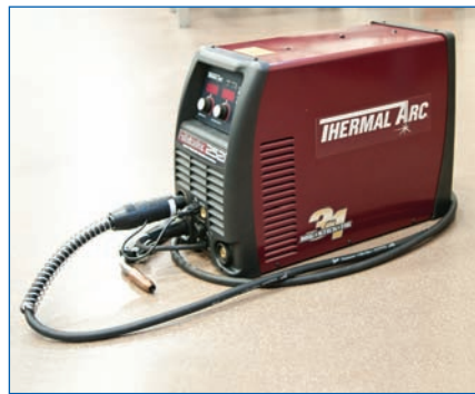
Three process (SMAW, GMAW, GTAW) welder donated by Thermadyne Industries, Inc.
