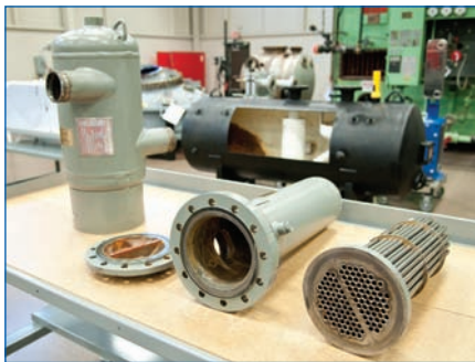
Foreground left and right: Air separator and U-tube heat exchanger donated by ITT Corp. Background: Cut-away deaerator donated by Ware, Inc.
