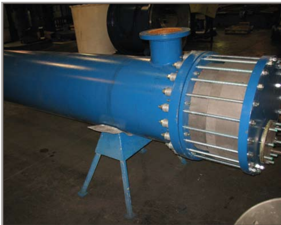
Tube and Shell Heat Exchanger, Courtesy of SGL Carbon Technic LLC.
