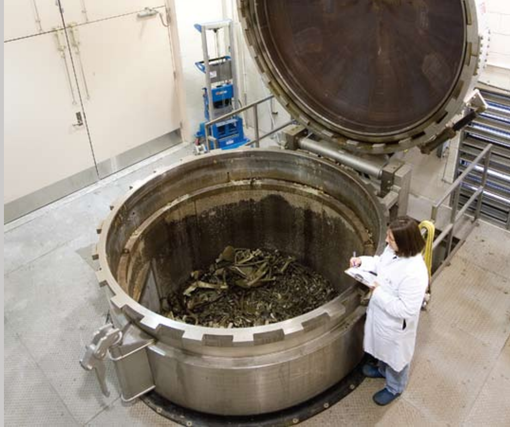
RIGHT & MIDDLE BOTTOM: Christy Ammons, ODA Veterinary Pathology Assistant, inspects the tissue digester. MIDDLE TOP: A pathologist dissects animal tissue. FAR RIGHT: Clayton Steam Generator
