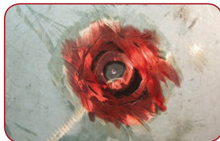
Figure 5. Head spin hole plug weld after the application of the penetrant.
