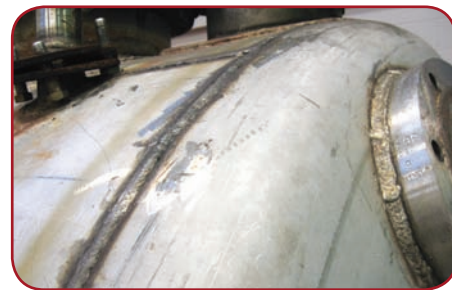
Figure 3. The knuckle of a stainless steel pressure vessel head that has been in service.
