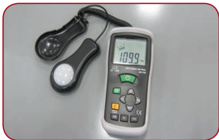
Light meter showing 109.9 footcandles of light.
