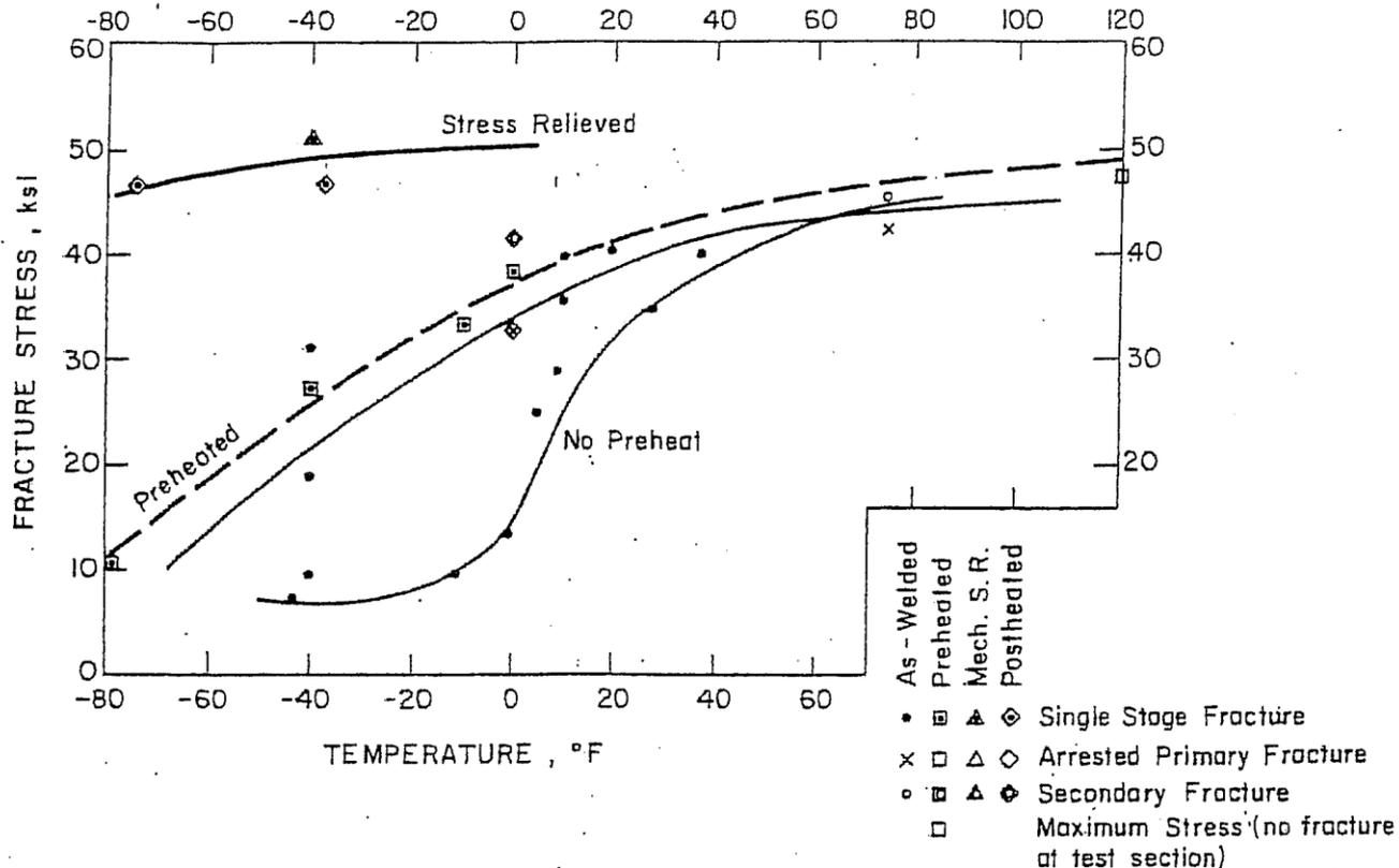
FIG. 8.12 Fracture Stress Variation with Temperature in A212 Grade B Wide-Plate Weldments Notched After Welding.
