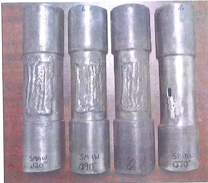
OD: Carbon Steel (P1) SMAW (Stick) process with E 7018 - 3/32" was used on these samples. The Weld Progression was Uphill. On all 4 of these samples the Welder Burned-thru the base metal, as the samples got thinner, the Burn-thru was more frequent.
