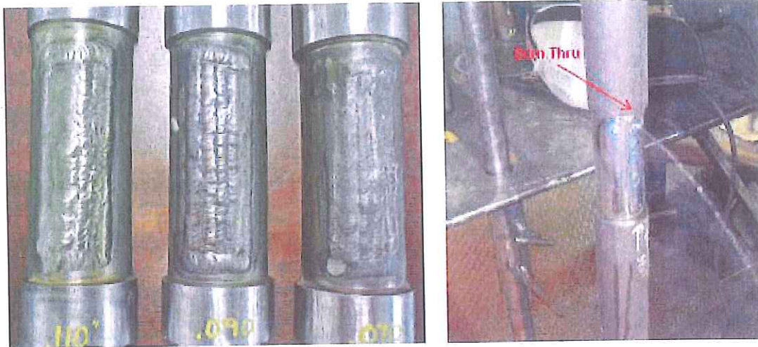
OD: 1-1/4 Chrome (P4), SA 213 T11: Superheat Tube Simulation (with Water in the Tube). GTAW (TIG) process with ER 80S B3- 3/32" was used. The Weld Progression was Uphill. Welder Burned-thru the base metal once on the .090" sample and multiple times on the .070" sample.
