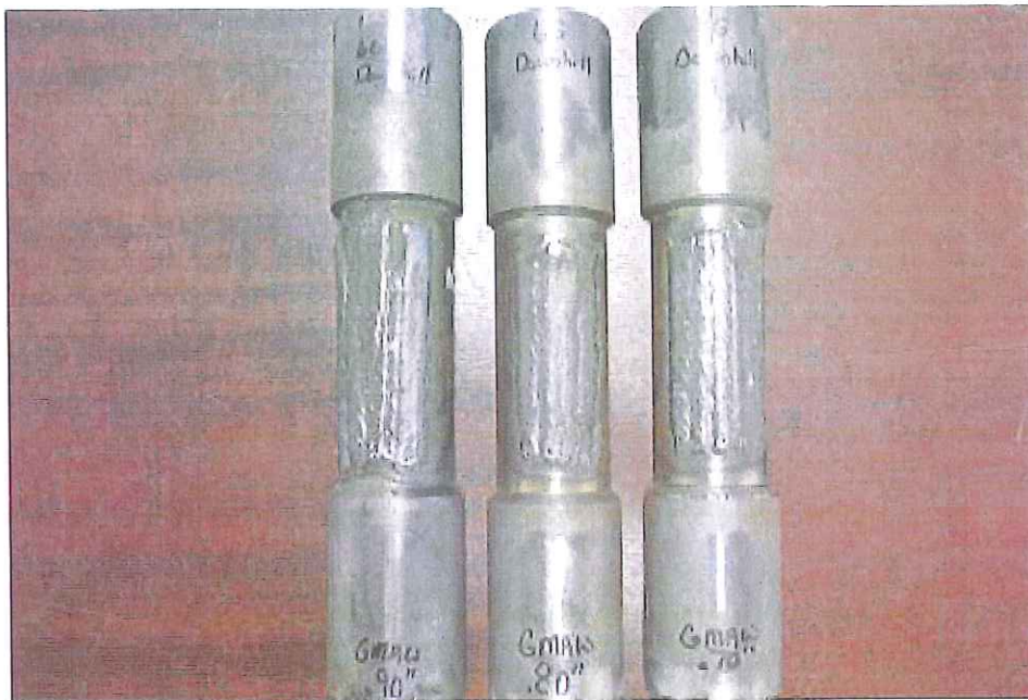
OD: Carbon Steel (P1), GMAW (MIG) process with E 70 S2 - .035" Wire was used on these samples. The Weld Progression was Downhill. Uphill is not recommended. On all of these samples the Welder had very minimal Melt-thru on all thicknesses of the base metal. The GMAW Process requires the base metal to be very clean. When applying Weld Build Up on Tubes of approximately .120" and below, GMAW (MIG) is the preferred method for Weld Build UP.
