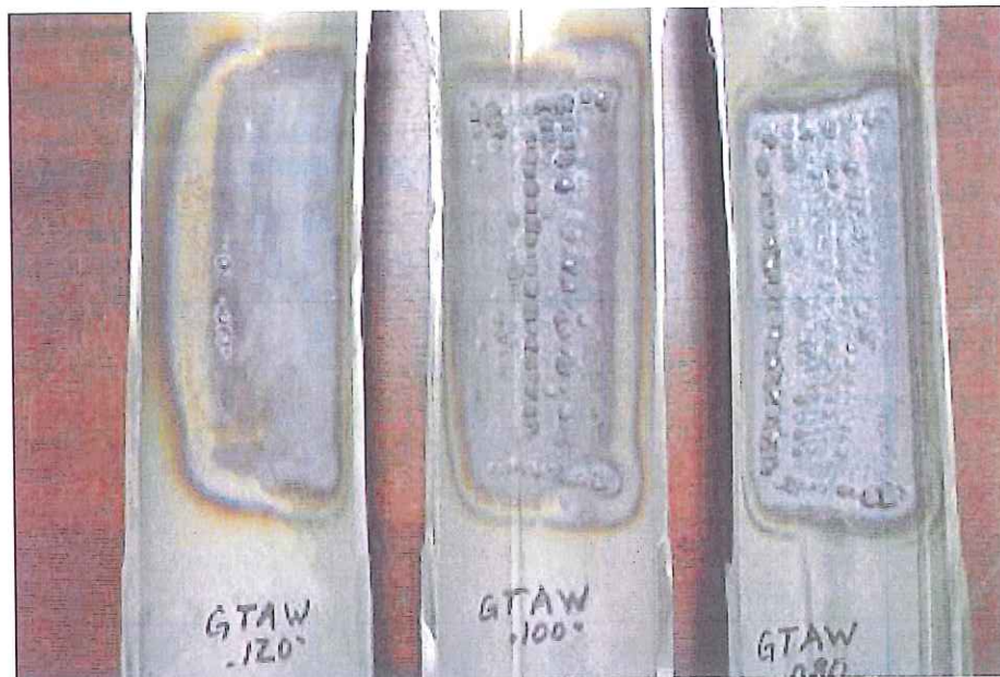
ID: Stainless: The Melt-thru on the .100" & .080" thick samples was excessive and "Sugared" (oxidized) the ID of the Tube. This is because the ID of the Tube is not accessible to use a Backing Gas such as Argon to shield the base metal or weld area.
