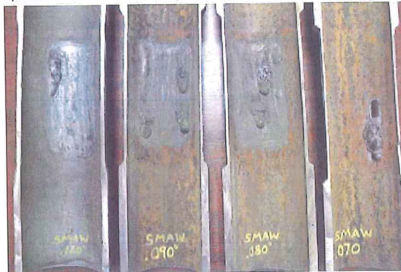
ID: Carbon Steel (P1) The Burn-thru that you see here is not "Melt-thru" it is "Burn-thru." Holes were actually burned in the base metal and filled back up with the SMAW process as the Welder was welding. Note: .070" sample was too thin to Weld.
