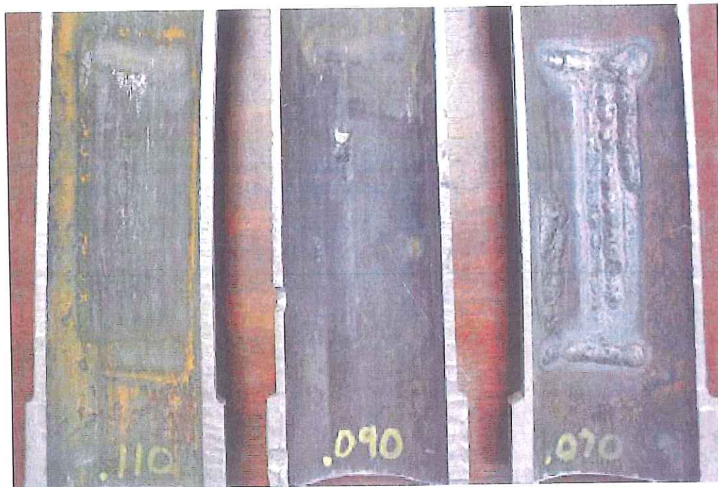
ID: 1-1/4 Chrome (P4), SA 213 T11 Superheat Tube Simulation (with Water in the Tube). With water in the Tube, there is little to no indication it is about to burn through the base metal. With the .070" Tube we had to let it cool 3 to 5 minutes between weld passes or between half a weld pass.
