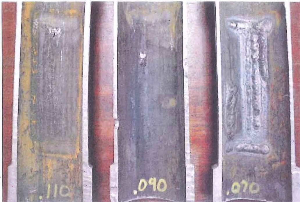
ID: 1-1/4 Chrome (P4), SA 213 T11 Superheat Tube Simulation (with Water in the Tube). With water in the Tube, there is little to no indication it is about to burn though the base metal. With the .070" Tube we had to let it cool 3 to 5 minutes between weld passes or between half a weld pass.
