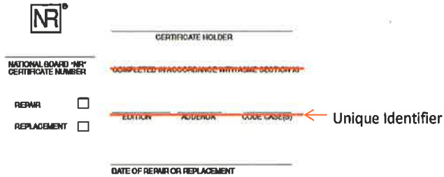
FIGURE 5.7.5-f REQUIRED MARKINGS FOR NUCLEAR REPAIRS OR REPLACEMENTS
