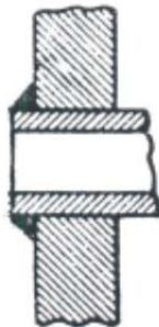
ROLLER EXPANDED USING STRAIGHT ROLLER & SEAL WELDED - SEE FIGURE S1.2.9.2 FOR DETAILS
