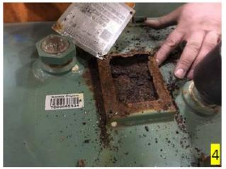
**Proposed text addition:** Refurbishers may need to temporarily physically remove the nameplate of ASME pressure vessels (LPG) that are mounted on a bracket and raised from the vessels surface to remove all coatings and to inspect and measure for corrosion under them.
