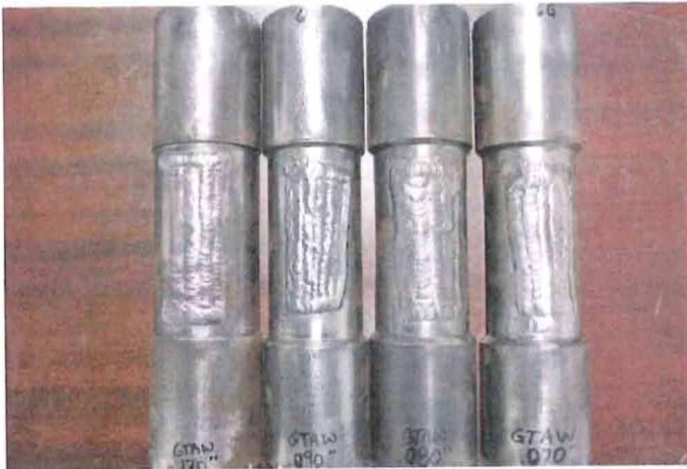
OD: Carbon Steel (P1), GTAW (TIG) process with E 70 S2 - 3/32" was used on these samples. The Weld Progression was Uphill. On all 4 of these samples the Welder Melted-thru the base metal, as the samples got thinner, the Melt-thru was more frequent and excessive.
