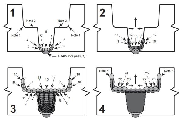
**Note 1** – The excavation shall have rounded corners to prevent lack of fusion defects. In these locations it is recommended to use a smaller diameter electrode (such as 3/32 in.(2.4 mm)) to ensure acceptable fusion.
