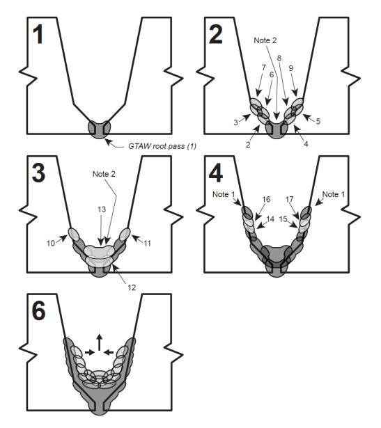
**Note 1** – Where the excavation may pose challenges with electrode access, it is recommended that the fill passes in immediate contact with the machined excavation be restricted in height as the weld repair is performed.
