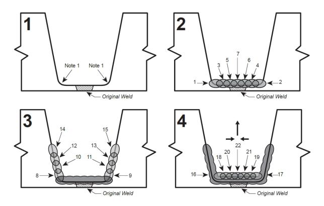
**Note 1** – The excavation shall have rounded corners to prevent lack of fusion defects. In these locations it is recommended to use a smaller diameter electrode (such as 3/32 in.(2.4 mm)) to ensure acceptable fusion.
