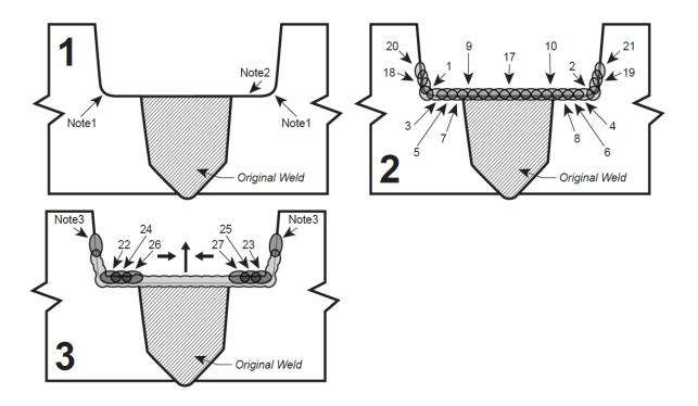
**Note 1** – The excavation shall have rounded corners to prevent lack of fusion defects. In these locations it is recommended to use a smaller diameter electrode (such as 3/32 in. (2.4 mm)) to ensure acceptable fusion.
