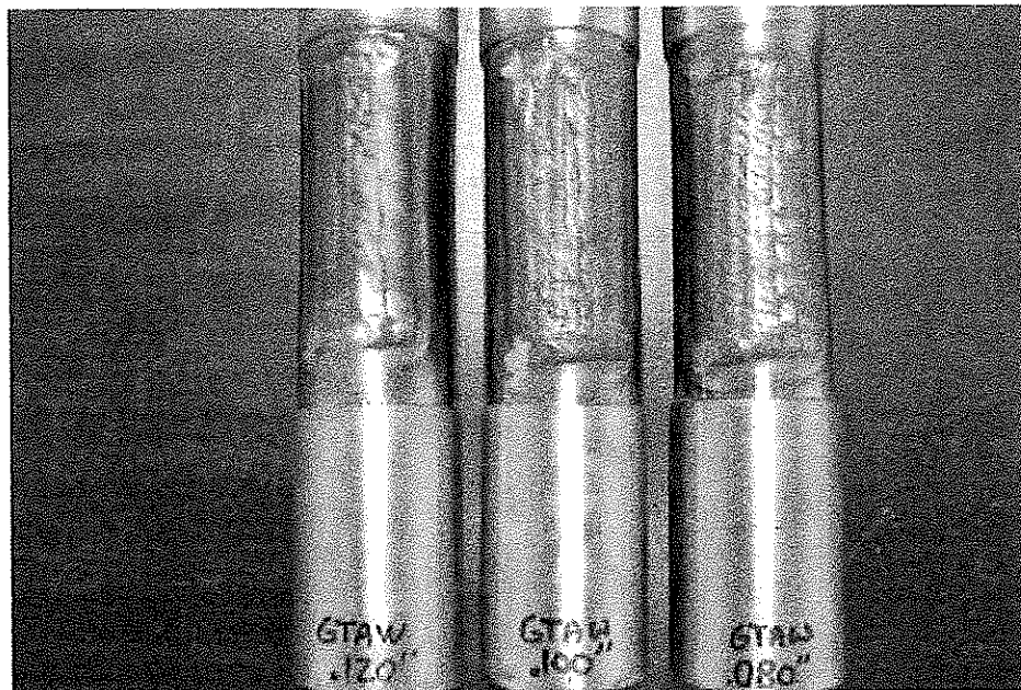
OD: Stainless: GTAW (TIG) process with E 316L - 3/32" was used on these samples. The Weld Progression was Uphill. On all 3 of these samples the Welder Melted-thru the base metal, as the samples got thinner, the Melt-thru was more frequent and excessive.
