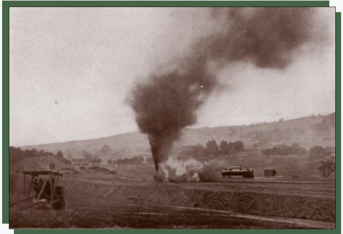
◆ The radial-stay boiler at the moment of failure. Escaping steam and water through the ruptured crown-sheet mingled with smoke from the stack and formed a cloud several hundred feet in height, completely enveloping its surroundings.
