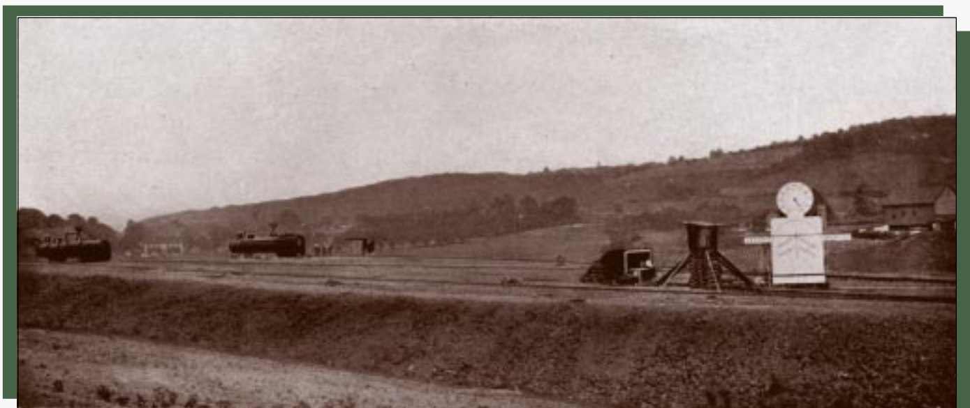
◆ General view of low-water testing grounds, showing location of boilers with reference to each other, shelter for the operating staff, elevated fuel-oil tank, and large display board for indicating to guests in the pavilion the boilers’ water levels and steam pressures during the tests.
