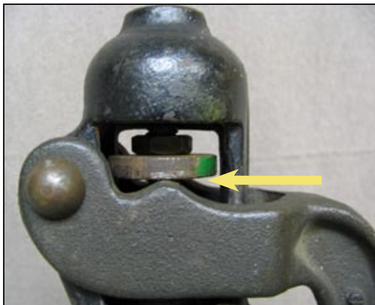
Insufficient clearance between the lift lever and the lifting nut.
