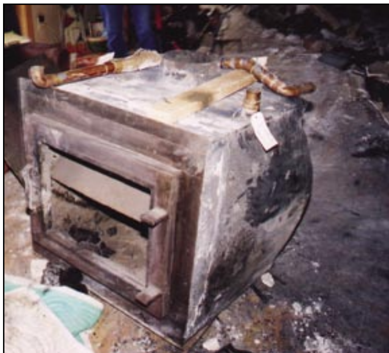
Front of wood boiler removed from window with only two water connections. Note lack of relief valve. ▼
