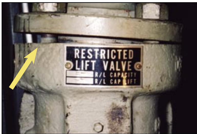
Improper assembly of the bonnet to the body.
