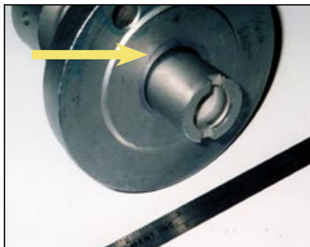
Excessive clearance between the disk holder and the guide.
