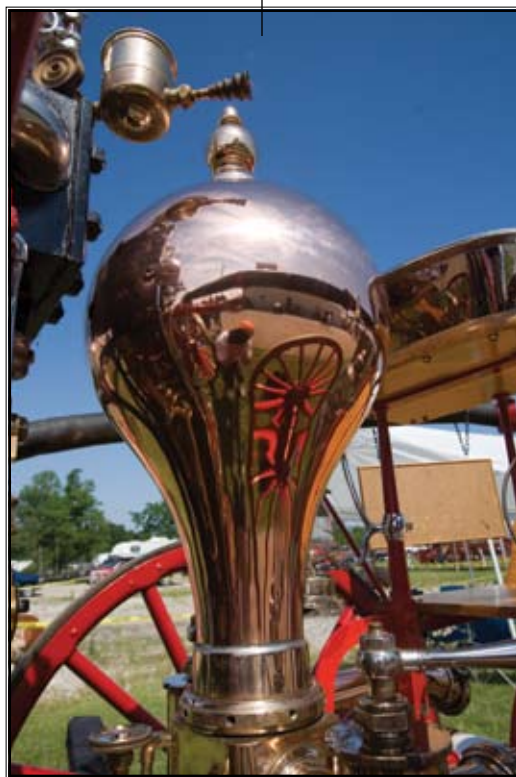
Copper balloon air chamber found on a steam fire engine.
