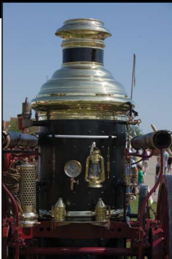
Watertube boiler of an 1892 Ahrens.
