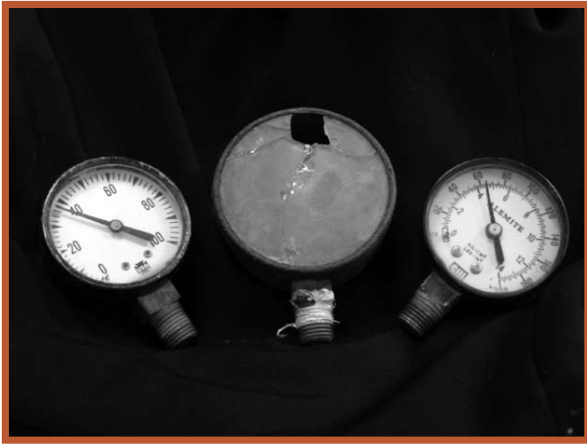
Three deficient pressure gages. The one in the center is broken. The other two indicate pressure, though there is no pressure source.
