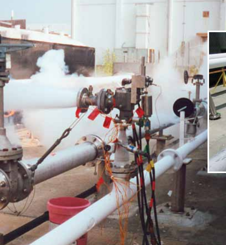
Valve tested with low-temperature fluid.
