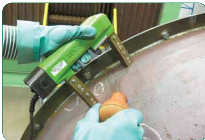
MT examination of the longitudinal seam on an inservice boiler.
