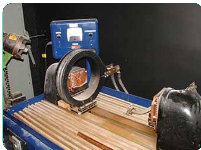
A stationary magnetic particle examination system set up for longitudinal and circular magnetization using wet fluorescent particles.
