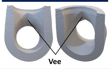
Cracks in welds due to poor geometry, proximity to crotch, inferior performance
