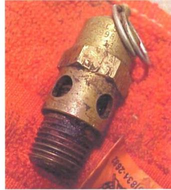
B. On receipt inlet of 125 psig valve is clogged with debris
