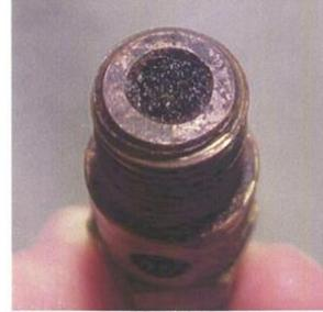
C. After test debris is blown through valve, rubber seat of valve is missing.
