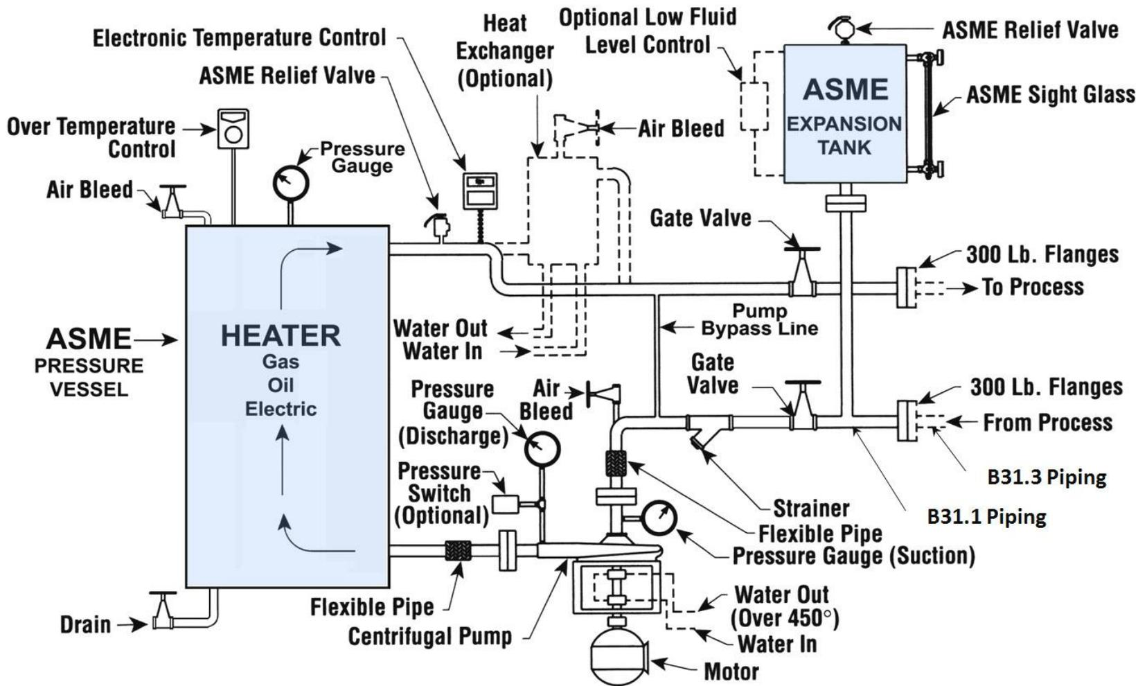
**TYPICAL ASME HOT OIL HEAT TRANSFER PRESSURIZED SYSTEM (OVER 15 PSIG)**
