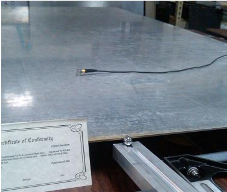
Figure 1. Rolling Ball Impact Calibration Setup.
