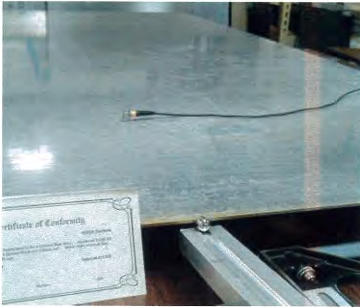
Figure 1. Rolling Ball Impact Calibration Setup.
