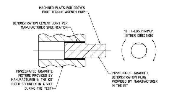
NOTE: THIS DEMONSTRATION APPLIES TO PLUGS OF ALL DIAMETERS AND LENGTHS.
