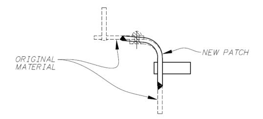
VIEW SHOWING NEW PATCH ALIGNMENT WITH ORIGINAL MATERIAL
