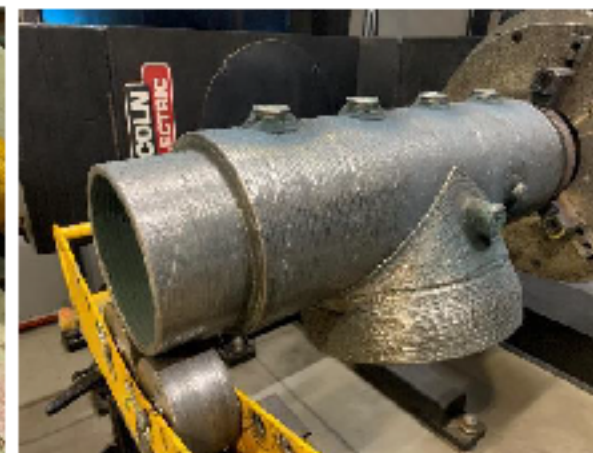
Piping components being printed at Lincoln Electric Additive Services
