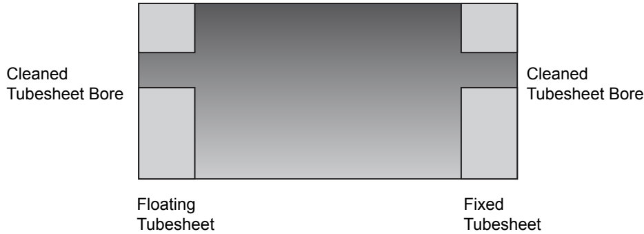
FIGURE S3.5.6-a CLEANED AND PREPARED TUBESHEETS
